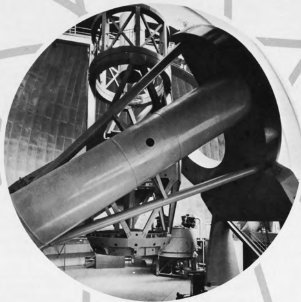
The 200-inch Hale telescope on Mt. Palomar shown pointing directly overhead. —Mt. Wilson and Palomar Observatories
