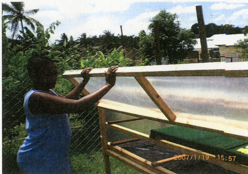
Trainee using a solar drier for fruit drying
